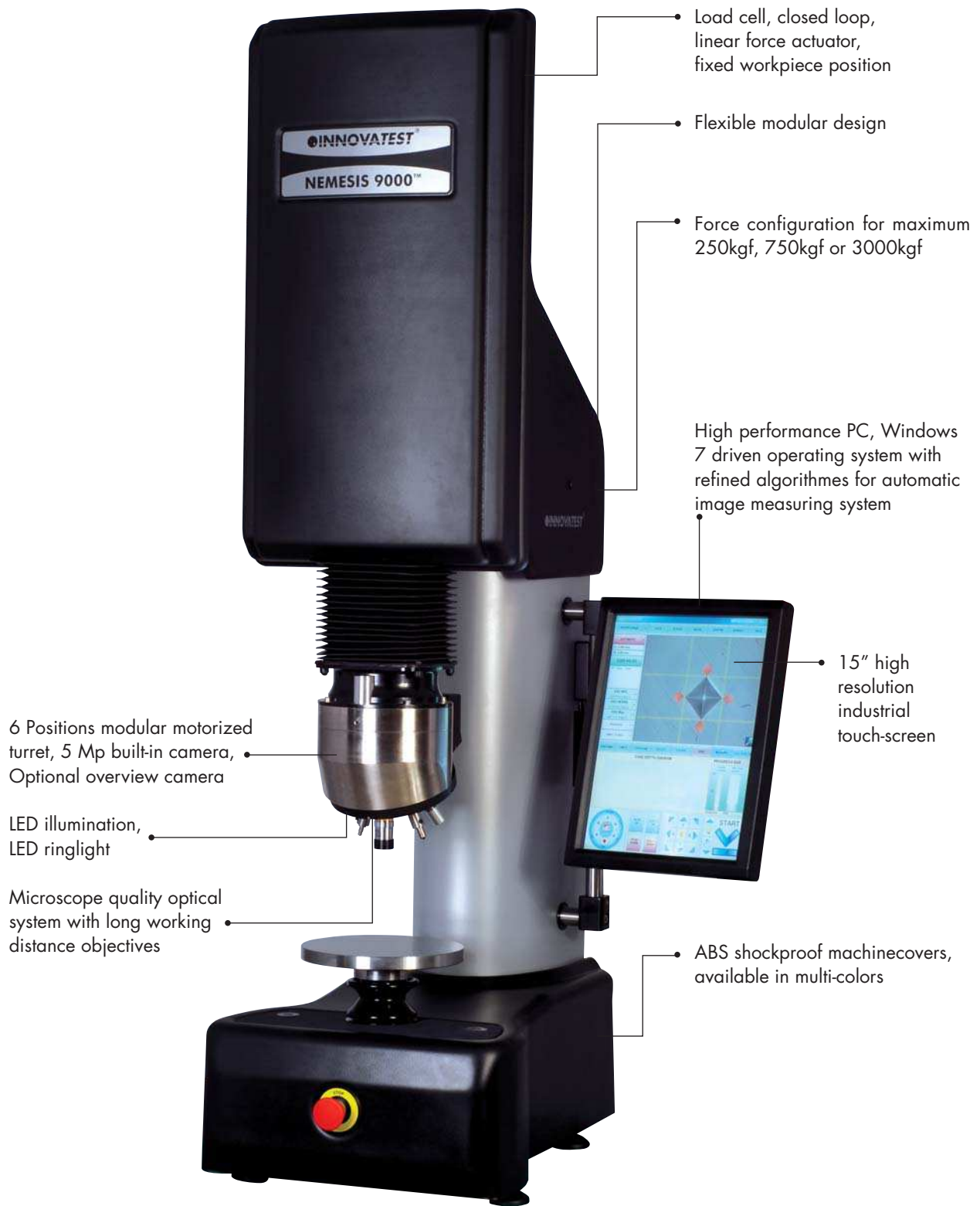
NEMESIS 9000™ SERIES 0.5KGF TO 3000KGF, 6 POSITION MOTORIZED TURRET
